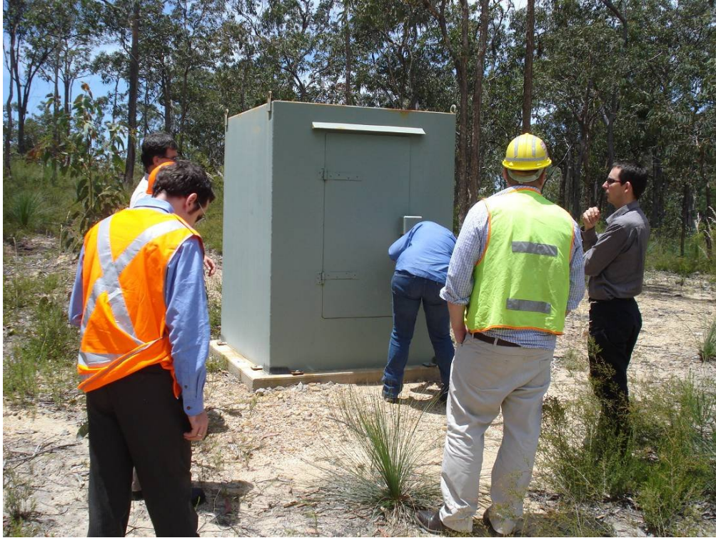
Plate 1 – Enclosure which contains the vibration monitors and piezometers / extensometers.
