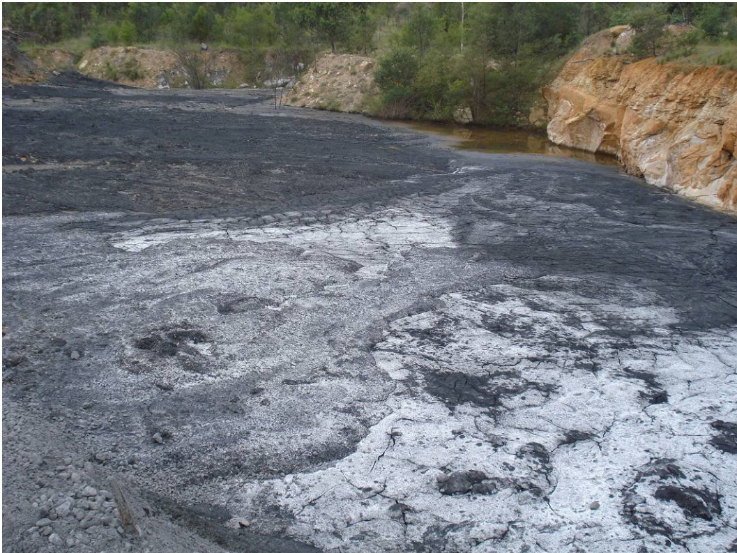
Plate 28 – Coal fines are pumped to voids within the rejects emplacement area. The water drains back into the underground.
